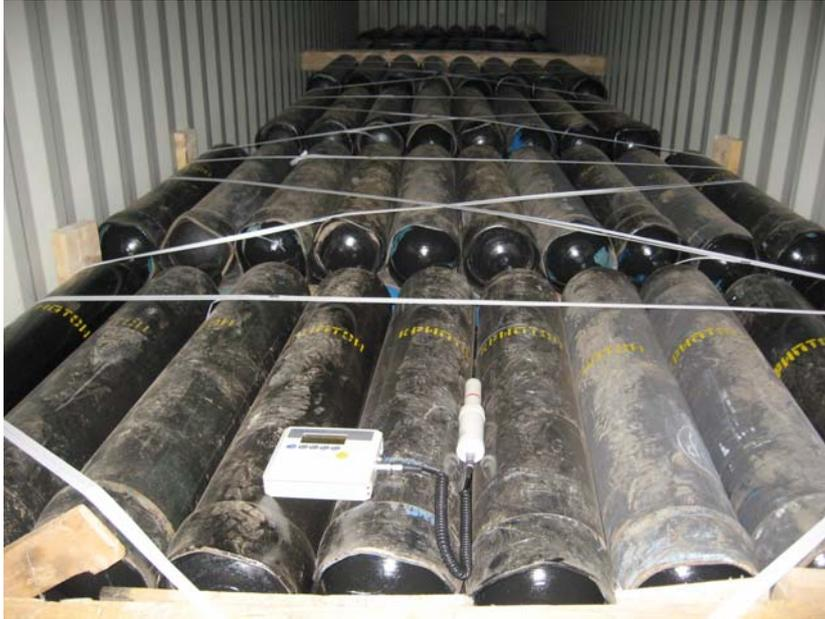
**Fig. 1. Cargo of steel cylinders containing pressurized krypton gas, with the dose rate meter in measurement position**
