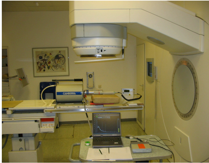
Fig. 2: Complete experimental setup, showing gamma detector (left) and dose rate meter (right) on the treatment couch top, plus spectrometer hardware in front.
